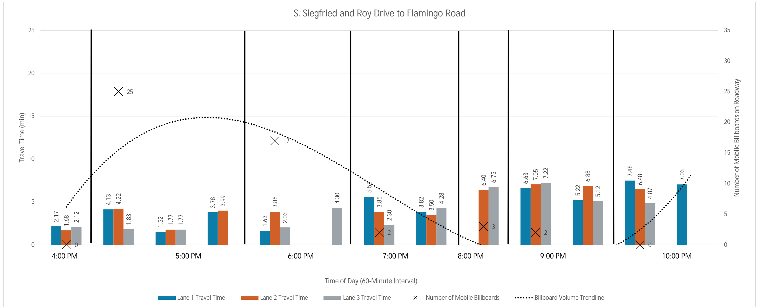
Graph G.5.80 – Southbound Travel Time in 60-Minute Intervals by Lane With Mobile Billboard Counts and Trendline Observed Between S. Siegfried and Roy Drive and Flamingo Road on Saturday, June 25, 2022 (Non-Holiday Weekend)
